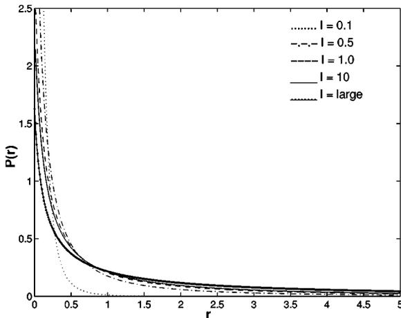
FIG. 2. The probability distribution  $P(r;l)$  in the case of the white noise disorder given by Eq. (3) and a pure imaginary mismatch ( $\phi_r=0$ ) for different lengths of the sample. The line joining the dots is the analytic result for  $P(r;\infty)$ . The amplification parameter is  $A = -1$ .
