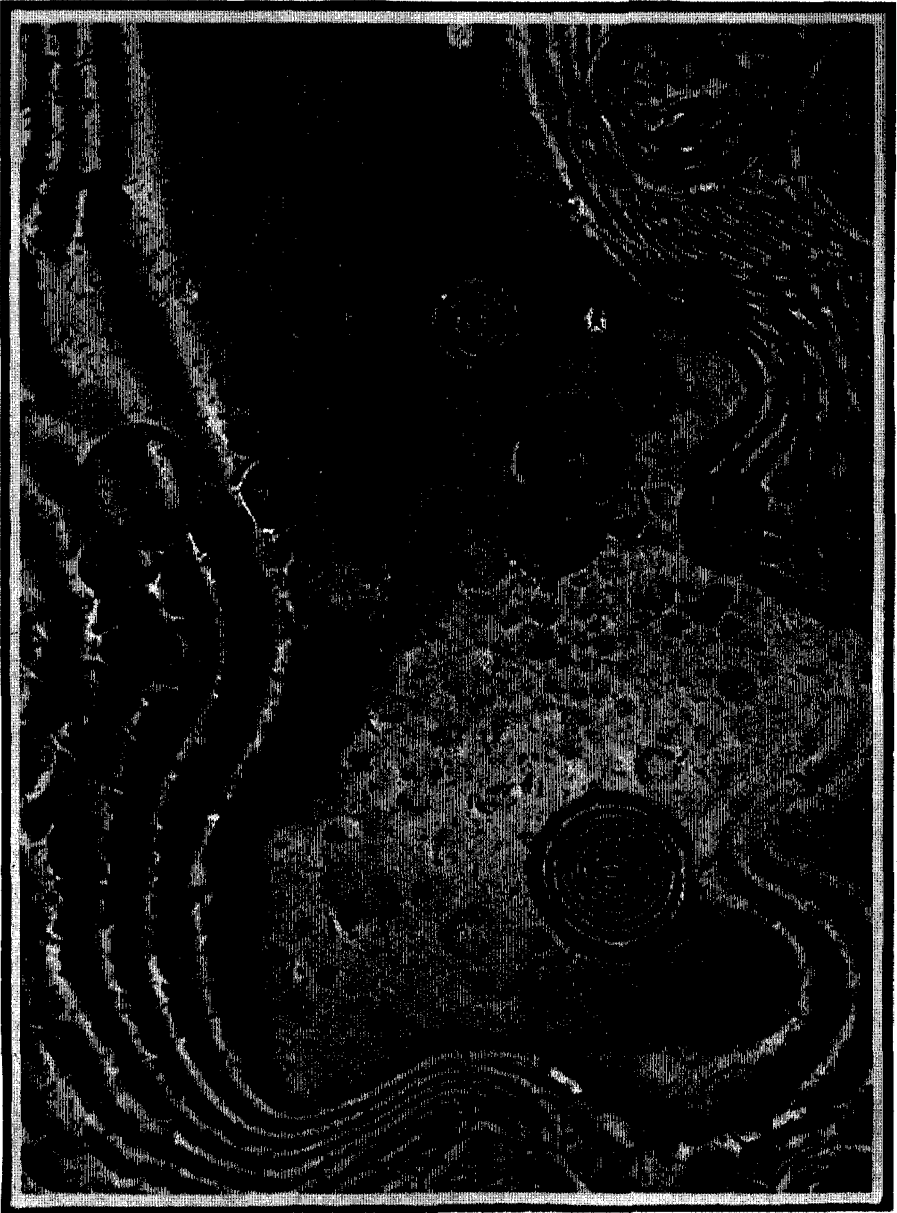
Figure 4. Photomicrograph of decomposed glass in transmitted monochromatic light, showing sharply defined fringes due to intruding air films.
