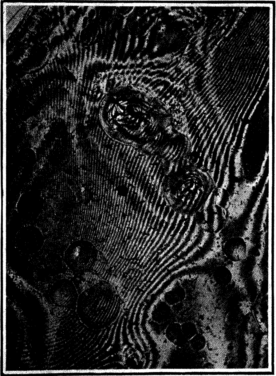
Figure 5. Photomicrograph of decomposed glass in transmitted light, showing cavities and fringes due to intruding air films.
