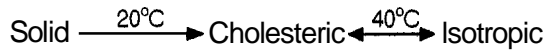
Figure 3.1: Showing the phase sequence and transition temperatures of the three pure compounds used in the experiments.
