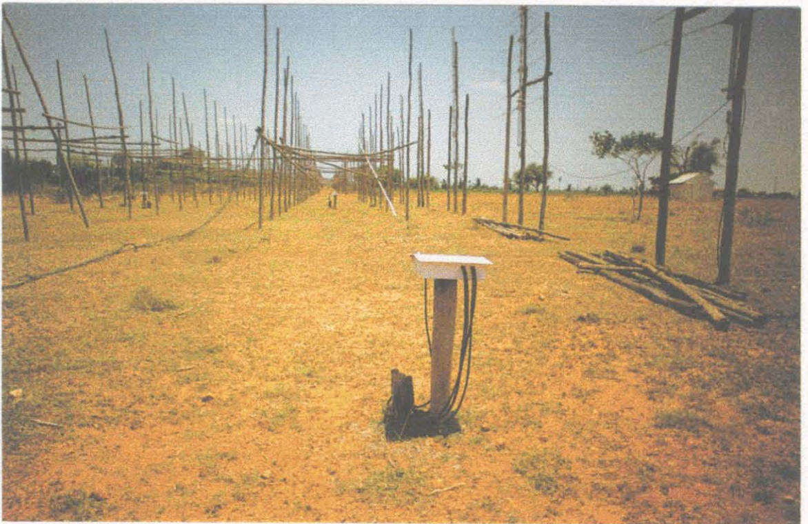
Figure 33 The fury of Mother Nature and low-frequency radio telescopes! A wild storm with intense lightning, strong winds and heavy rains swept through Gauribianur on the 30th May 1995. It left behind a trail of destruction as demonstrated by these two photographs. The last section of the east arm is shown here. A lone amplifier box stands in the midst of uprooted poles and hanging dipole wires. This damage was subsequently repaired by the observatory team at Gauribianur and the telescope was made as picture perfect as in Fig 32.
