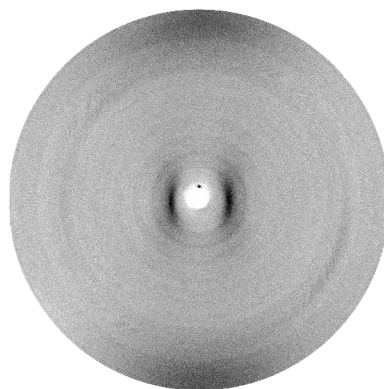
Figure 4.45: The X-ray diffraction pattern of a binary mixture with 60 mol% of CP6B at 50\text{ }^{\circ}\text{C} cooled in presence of 2.3 kgauss magnetic field.
