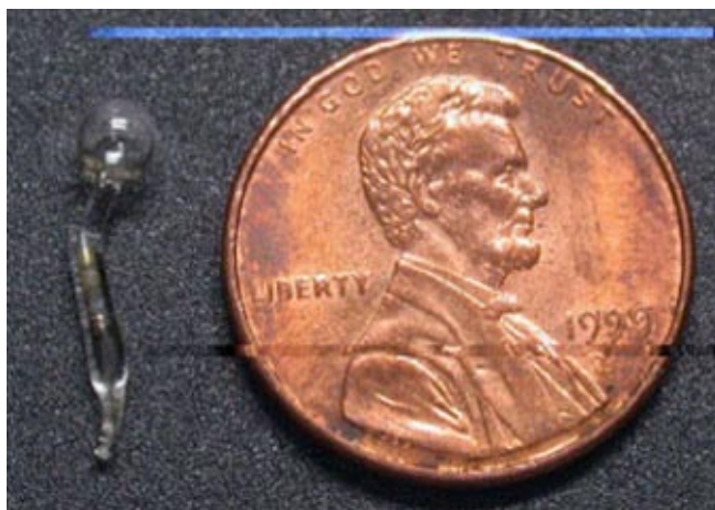
Figure 11. Cs-vapour microcell whose inner walls are coated with paraffin. Reprinted figure from M. V. Balabas et al., J. Opt. Soc. Am. B , Vol. 23, 1001 (2006) with permission from D. Budker.
