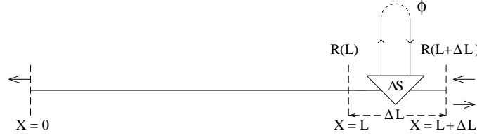
FIGURE 3.11: A schematic description of the ‘invariant imbedding’ method for a 1D conductor with random-phase reservoirs distributed uniformly along the length.
