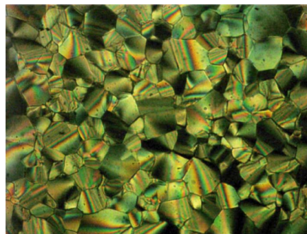
FIG. 1. (Color online) Polarizing optical micrograph of the composite 1% \text{HAuCl}_4/\text{HAT6} , on cooling from the isotropic phase.
