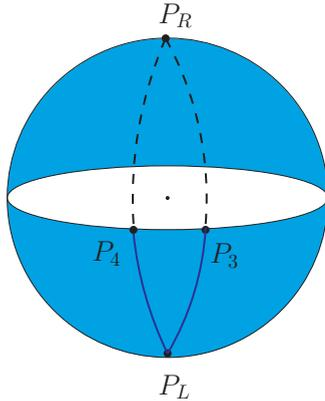
FIG. 2. (Color online) The path on the Poincaré sphere that determines the geometric phase. The angle  $\varphi_{34}$  between the linear polaroids determines the width of the lune on the Poincaré sphere and the geometric phase.
