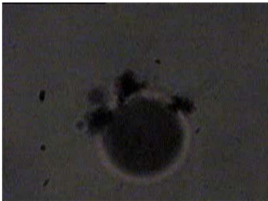
Figure 2: CNT bundles in the vicinity are attracted to the microbubble; they adhere to the surface of the bubble.
