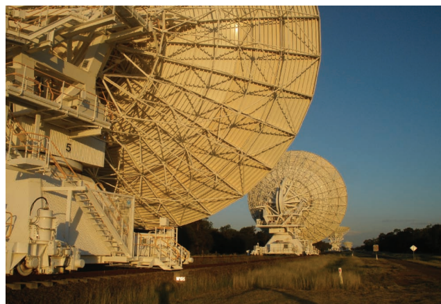
Figure 2. The ATCA. Displayed are several antennas on the east–west track pointing at a source near the horizon.
