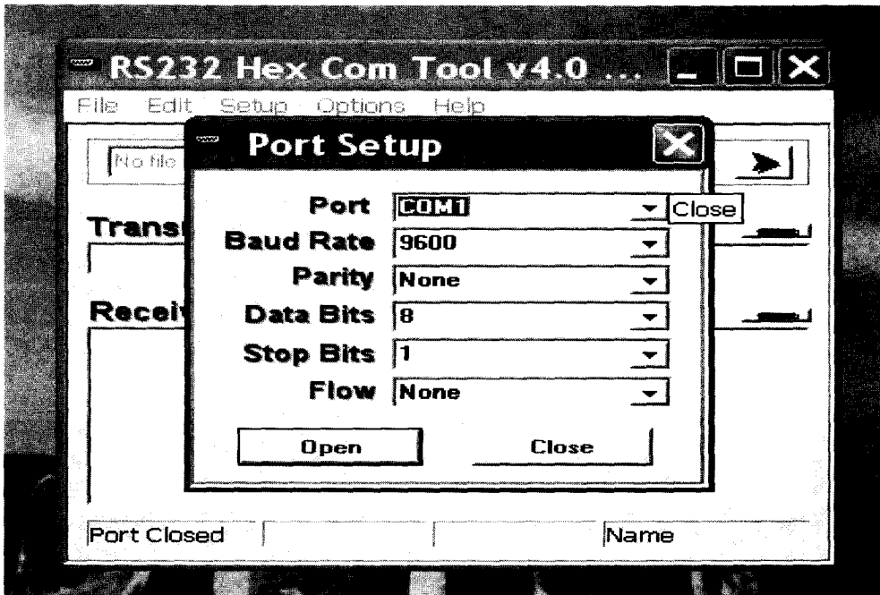
Figure 20: Selecting the Baud rate for local network using RS232 HEX COM tool – hyperterminal
