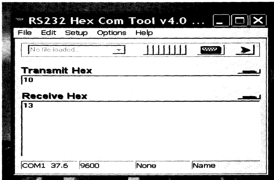
Figure 21: Example of sending the slave ID addressed 10H and receiving 13H as acknowledgement
