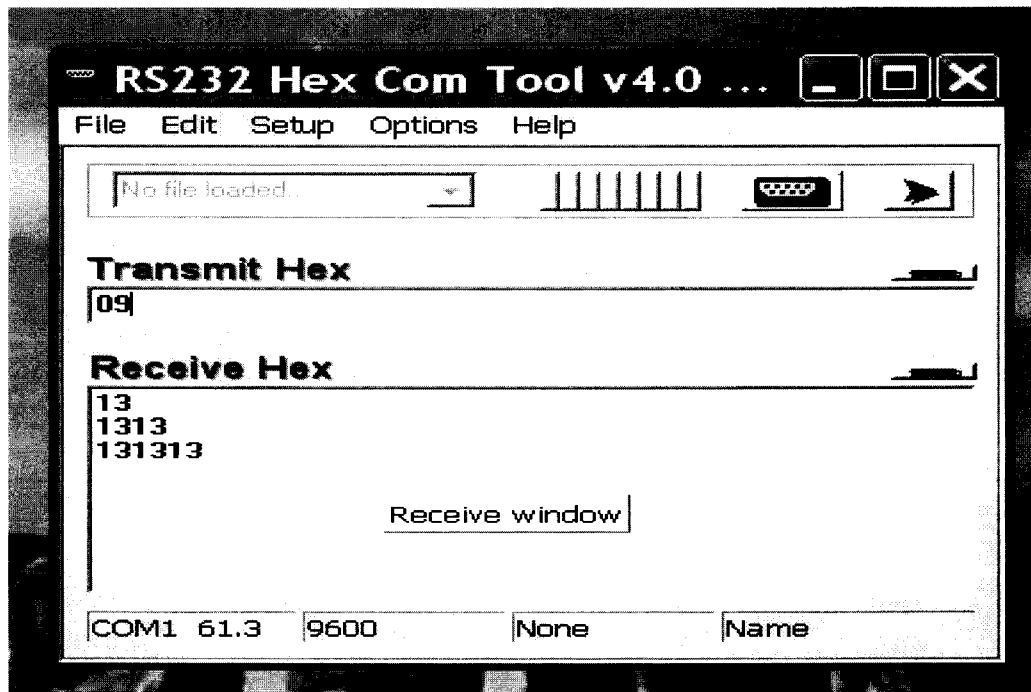
Figure 22: Demonstrating the ping_slave command – 13 is echoed back five times from the slave
