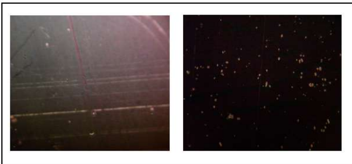
Fig 2.16: Optical textures exhibited in the nematic phase of pure E7
