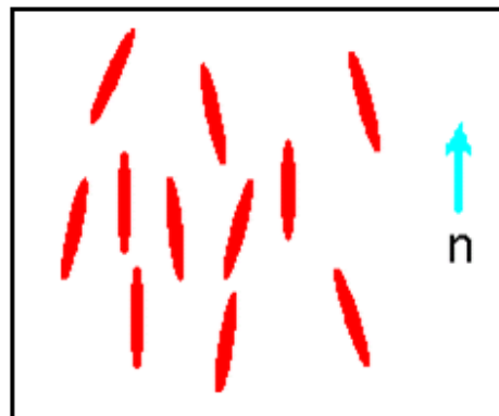
Fig 1.4 Molecular arrangements in the Nematic phase.
