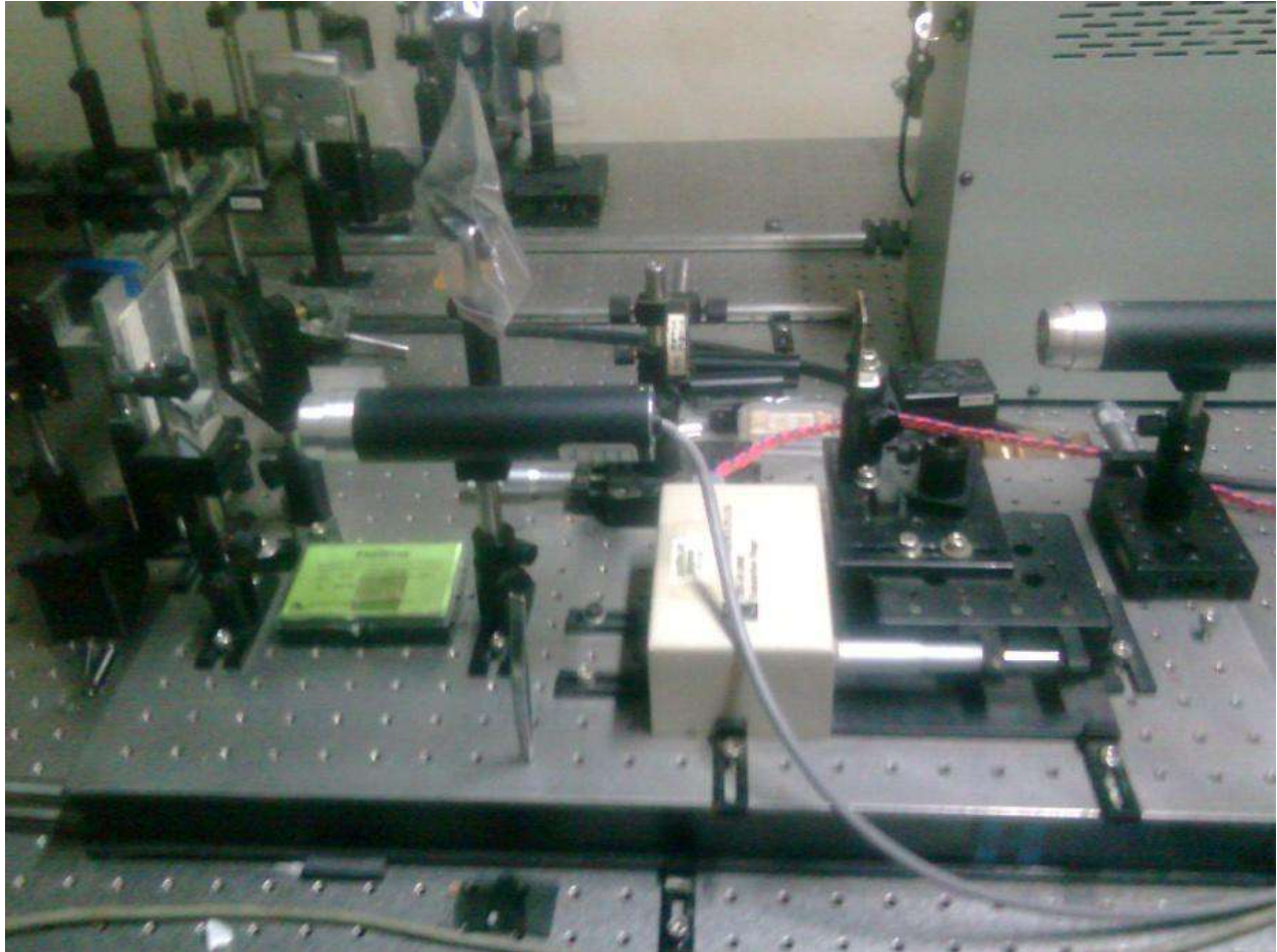
Fig 2.10: A photograph of the automated Z-scan setup used for our experiment.
