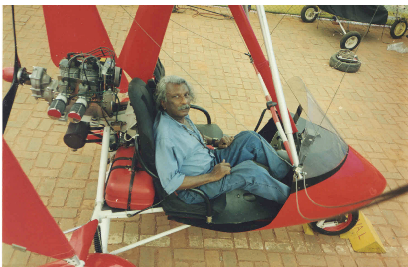
Fig. 2. A two-seater powered hang glider, especially designed for training. The two seats are side-by-side rather than in tandem (2000).
