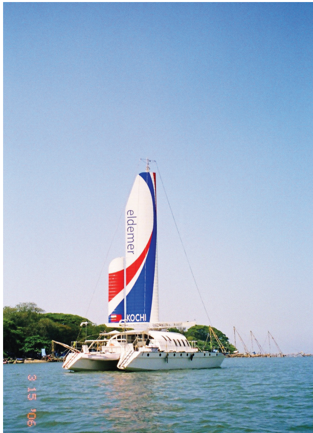
Fig. 4. Rad’s dream boat – Eldemer – double hulled boat with a sail resembling the wing of an aircraft (2005).
