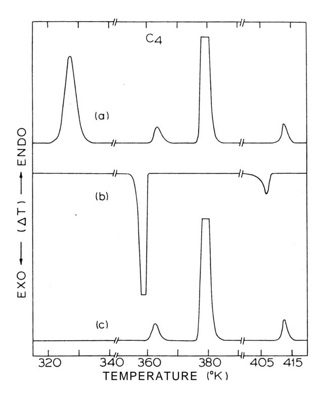
demonstrates this fact. (The small endethermic peak at ~360 K in the case of G<sub>4</sub> is due to a very weak solid-solid transition with an enthalpy comparable to that of the N-I transition. This is not seem in the cooling cycle but shows up in the reheating cycle.) OBOOA also exhibits a similar behaviour. 11
