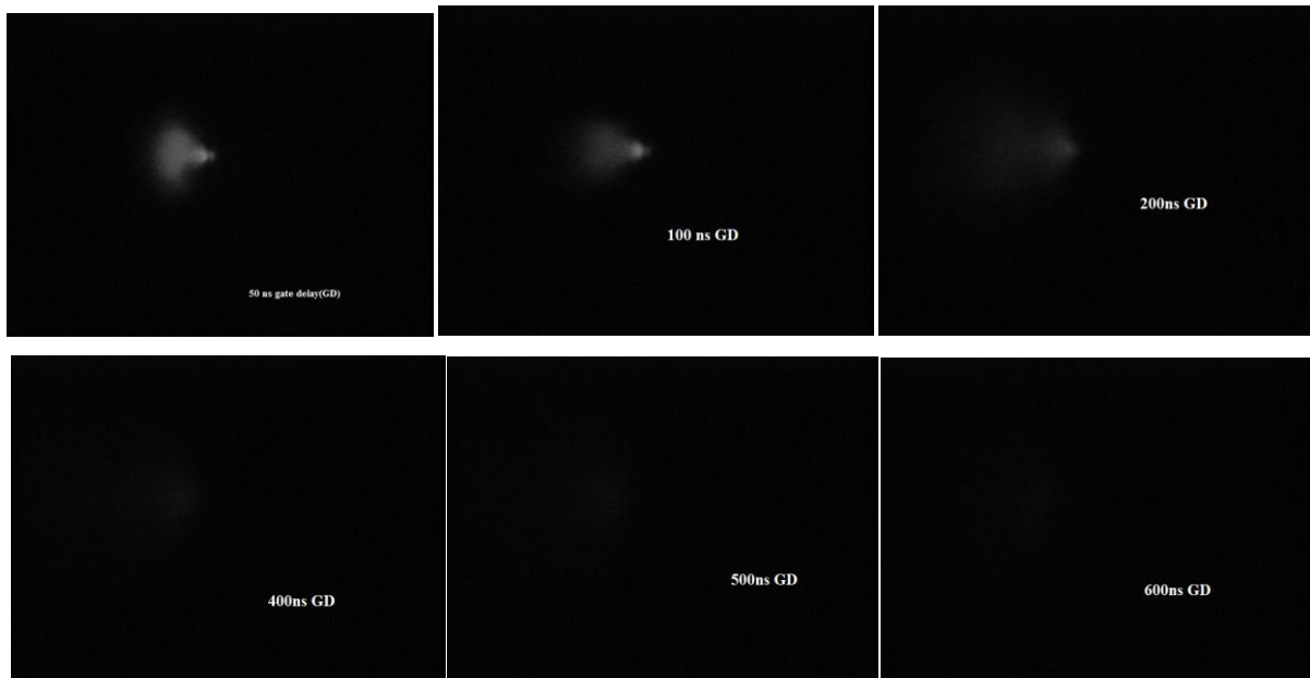
Figure5.1: ICCD photographs of visible emission from laser-produced copper plasma at 5\text{e-}6 Torr background air pressure
