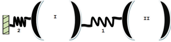
FIG. 1. (Color online) Schematic of the dual-spring-dual-cavity optomechanical system. The first cavity is attached to two springs.
