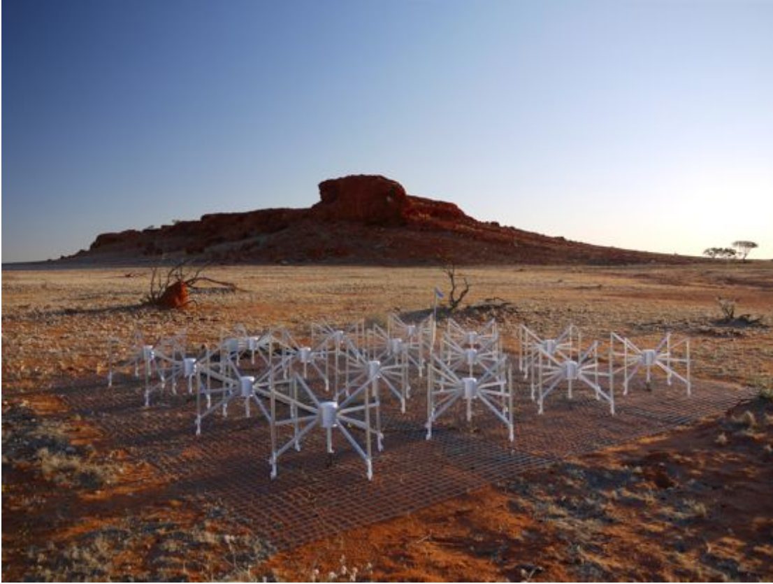
FIGURE 2.2: MWA tile with the 16 bow-tie dipoles in 4 \times 4 configuration on a 5\text{m} \times 5\text{m} steel mesh.
