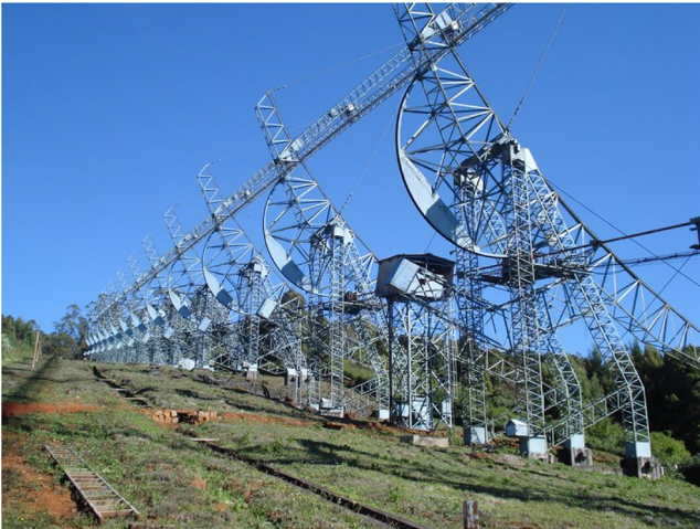
Figure 1. The Ooty Radio Telescope is an offset cylindrical paraboloid, 530 \text{ m} \times 30 \text{ m} in size. It is equatorially mounted. The Ooty Wide Field Array (OWFA) is an upgrade to the ORT, which digitizes the signals from every 4 dipoles along the feed line. These signals are then cross-correlated, leading to a very wide field-of-view interferometer. See text for more details.
