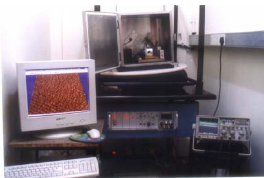
Figure 19. Picture of the STM built in Raman Research Institute (RRI)
