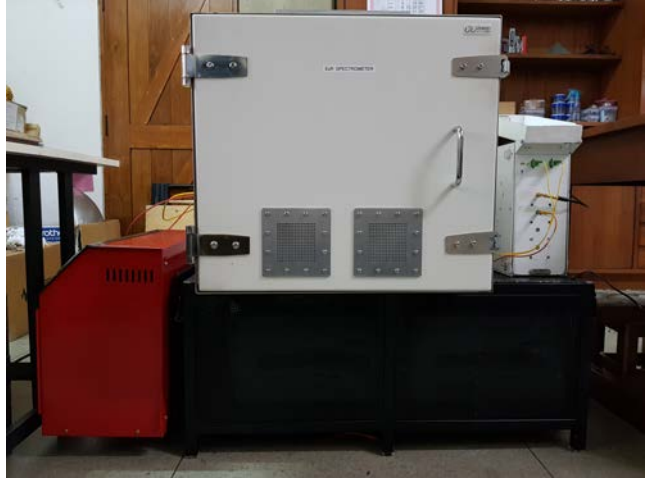
Fig. 6. The Digital Receiver is in the white colored shielded enclosure and the black painted shielded enclosure beneath the digital receiver houses the batteries. The analog signal conditioner is the unit to the right and the red unit to the left is the battery charger.
