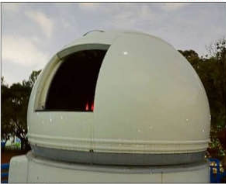
The 'Alice' dome set up at Raman Research Institute (RRI), Bengaluru, to stream a quantum key to a neighbouring building 50 metres away.
