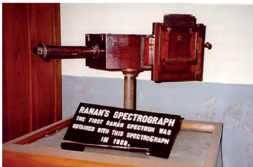
Above: The spectrograph used to record the first Raman Spectrum Below: The Raman Effect honored as the International Historic Chemical Landmark by the American Chemical Society in 1998
