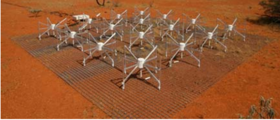
Figure 2.4: A tile of the Murchison Widefield Array (MWA) consisting of 16 crossed-dipoles placed on a wired mesh. Credit: MWA Collaboration.
