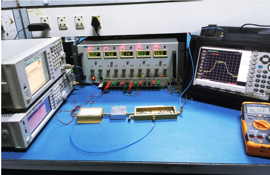
Figure 7. Test Setup of the Intermediate Frequency Processor in the Lab
