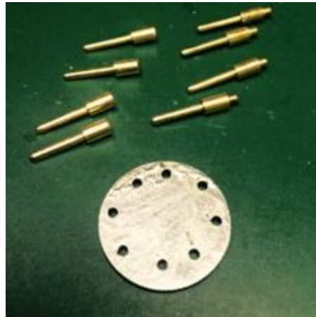
Fig. 3: circular plate with holes for mounting pins
