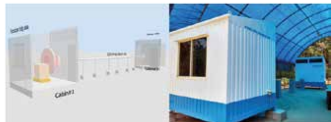
Fig. 12. 12m beam line – concept drawing (left) and the actual cabin installed
