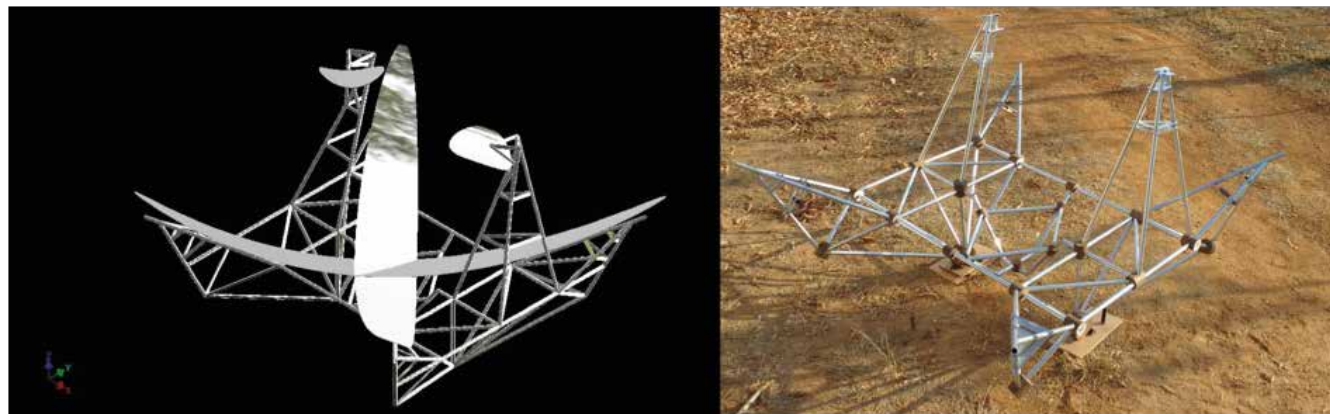
(Left) A CAD model view of the backup structure, with the mirrors set. (Right) A photo of the scaled-model of ELI, 2.3m x 2.3m, being built at Gauribidanur.
