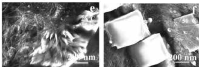
Self-assembled CNT-polymer hybrids consisting of cone-like and cube-like morphologies in 0.5 wt.% CNT dispersed aqueous triblock copolymer (P123) solution.
