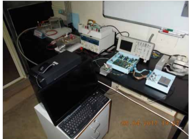
Fig. 11. Thermovac test setup for the high voltage unit
