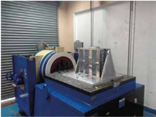
Fig. 9. POLIX detector undergoing vibration test on mechanical shaker
