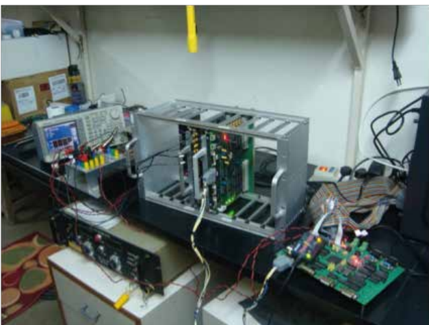
Fig. 10. Pre-engineering model of POLIX signal processing electronics
