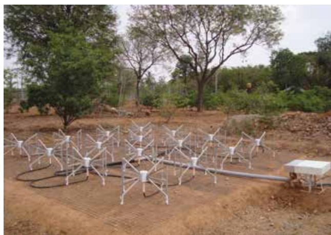
Figure 8. An array of 16 bow-tie antennas (MWA antenna tile) forming one of the elements of SWAN providing an enhanced BW of 250 MHz. The RF signal is down converted to
