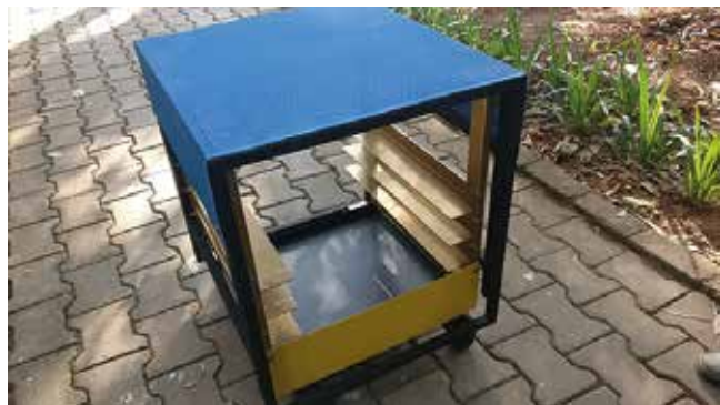
Figure 5. Chassis custom built with slots to house SWAN receivers
