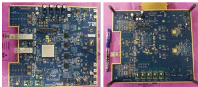
Figure 3. Top and bottom views of the signal processing platform built by the Electronics Engineering Group
