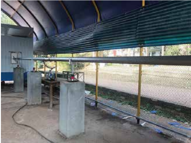
Figure 2. 12 m X-ray beamline with provisions for fine adjustments along both the vertical and horizontal directions.
