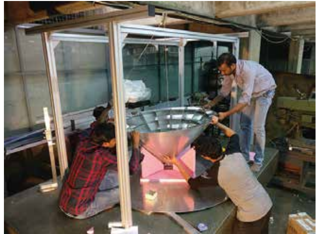
Figure 4. The SARAS antenna being carefully mounted on the SMA pin using a pulley. The pink Styrofoam support structure is clearly visible.
