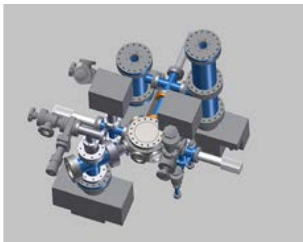
Figure 1. Schematic of the experimental set-up designed and being implemented at RRI. K and Na atoms will be collected into a dual species magneto optical trap (MOT) from two 2D-MOT sources, respectively. Thereafter, they will be magnetically transported to a vacuum cell with high optical access where the double degenerate cloud will be prepared and subsequently the molecules at ultra-low temperature will be formed.
