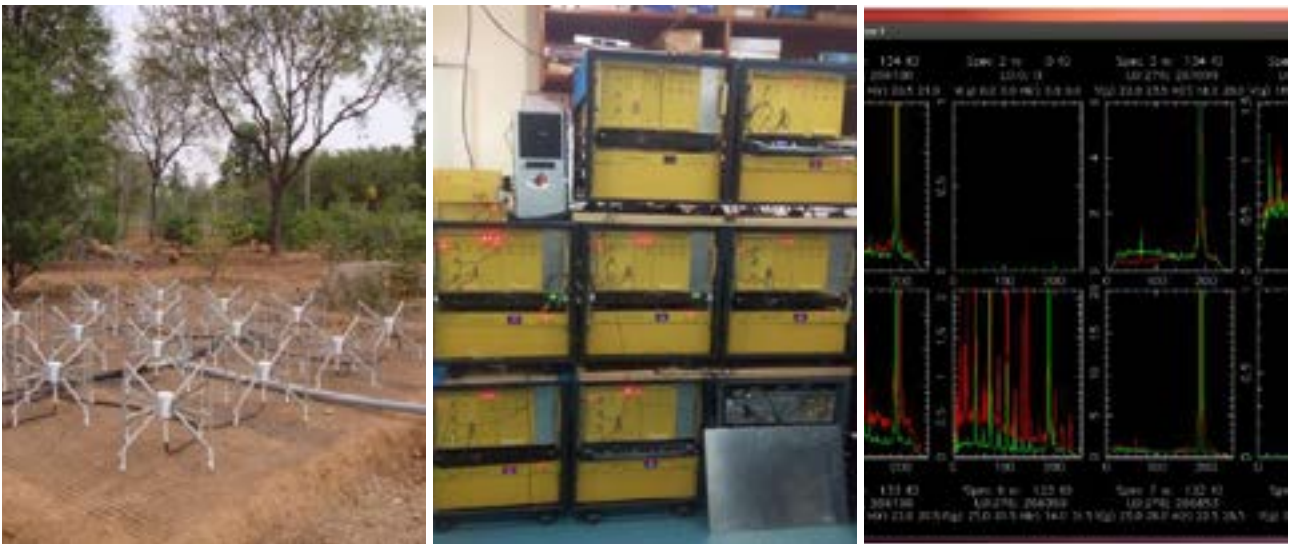
Figure 7. (Left) 4x4 bow-tie antennas forming one tile (Middle) Receiver systems kept ready after validation to shift to different academic institutions. (Right) Output spectra of different tiles at 140 MHz over a bandwidth of 14 MHz. Observe the presence of radio frequency interference
