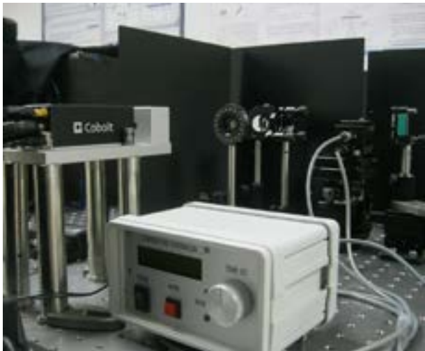
Figure 16. A photograph from the Quantum Information and Computing lab which shows a part of the single photon source that was used to establish the B92 protocol in the lab. The source has very high singles and pair generation rates. The average Coincidence rates is 0.56 MHz while the average pair generation rate is 17.1 MHz
