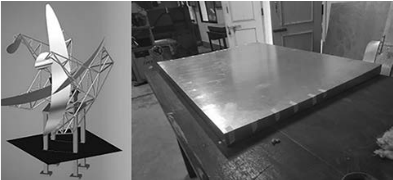
Figure. 5 (Left) A CAD model view of the entire telescope structure, with its base and the mirrors set on it. (Right) A photo of a prototype cylindrical panel for ELI of size 1.2m x 1m.
