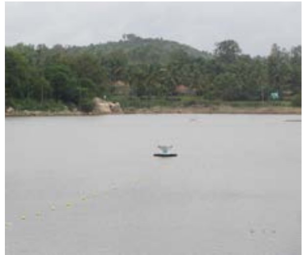
Figure 1. Conical monopole antenna being characterised for its impedance and radiation characteristics on the surface of water in Agara Lake situated near Banashankari, south of Bangalore. A small raft designed in-house was used to float the antenna and measurements were carried out in-situ while communicating with equipment at the antenna via optical fiber.
