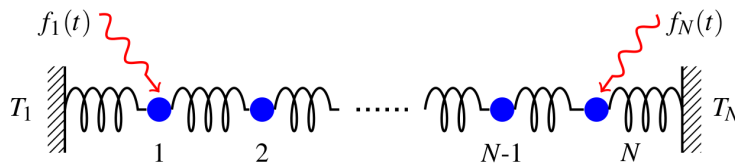
Figure 7.1: Schematic representation of a chain of oscillators connected to two nonequilibrium reservoirs which exert active forces f_{1,N}(t) on the boundary oscillators.
