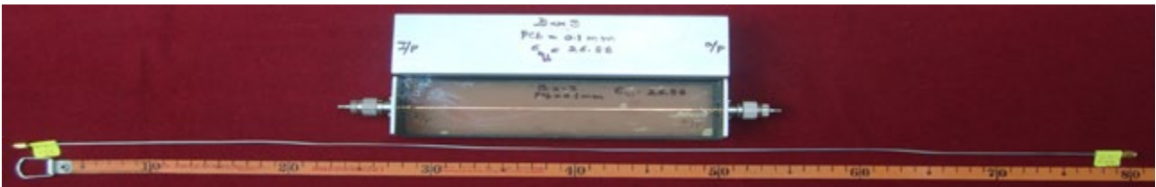
Fig. 7 RF transmission line of 205mm long on pcb = 0.1 mm thick + 10mm water is equivalent to 772 mm long RF cable.
