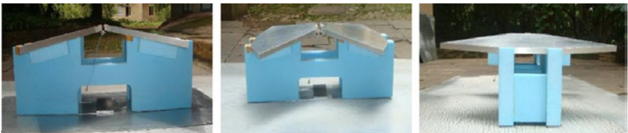
Fig. 1 Prototype of the reflector based shaped planar dipole antenna designed to operate in the band 120-360 MHz. Shown on the left, center and right are different views of the antenna.
