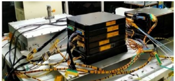
Fig.9a and Fig.9b Qualification Model Detectors and Electronics of POLIX
