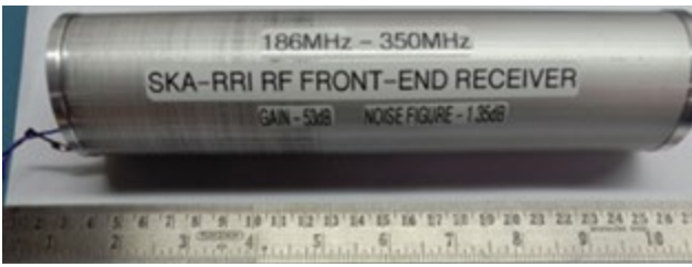
Fig.13 RF Front-End Receiver housed in a shielded cylindrical module of 50mm dia and 220mm length.
