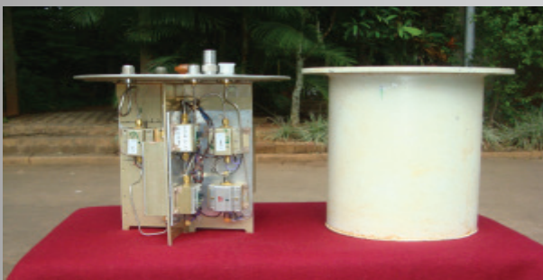
Figure 2: Two cylinders housing the front end electronics of the radio receiver.
