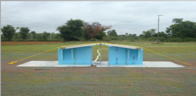
Figure1: The 30-90 MHz and 120-360 MHz antennas deployed in the Gauribidanur observatory to make sky observation.
