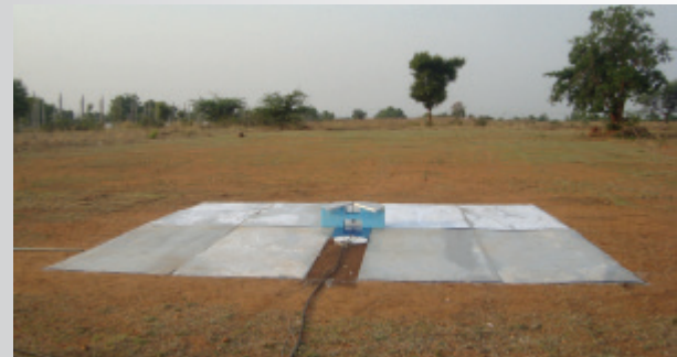
Figure1: The 30-90 MHz and 120-360 MHz antennas deployed in the Gauribidanur observatory to make sky observation.
