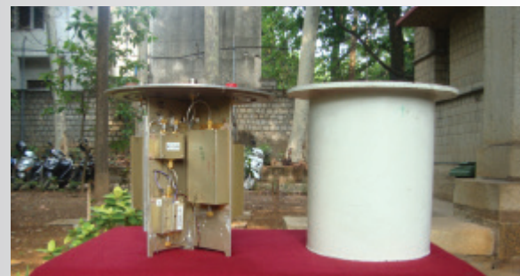
Figure1: The 30-90 MHz and 120-360 MHz antennas deployed in the Gauribidanur observatory to make sky observation.
