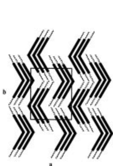
Figure 3. Schematic representation of the structure in the B_1 phase exhibited by compounds made of BC molecules ( p2mg symmetry).
